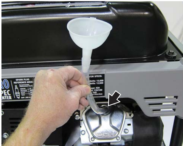
Figure 38 – Adding Engine Oil
