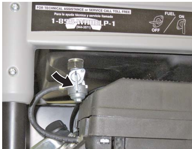
Figure 27 – Fuel Shutoff Valve in the ON Position
