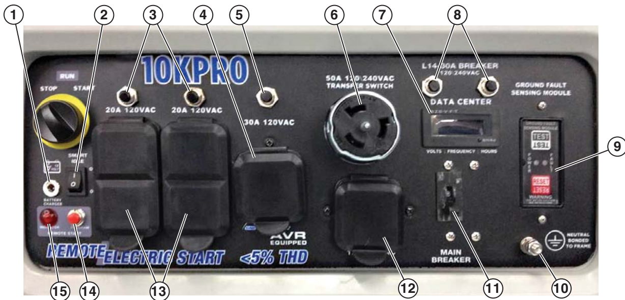
Figure 12 – Control Panel Features
