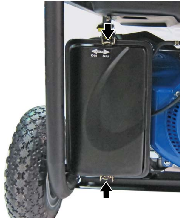
Figure 51 – Installation of Air Filter Cover
