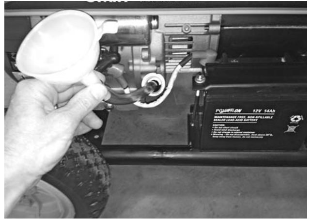
Figure 39 – Adding Engine Oil
